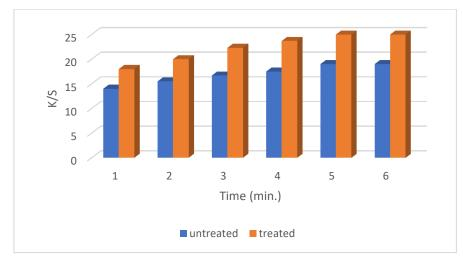
**Figure 8.** Effect of time on dyeing Wool Fibres by microwave method on color strength (K/S)
