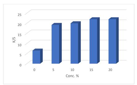
**Figure 5.** Effect of enzyme on the colour strength (K/S) for wool fibres dyed with madder natural dye
