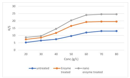
Figure 6. Effect of concentration of dye in dyeing processes
