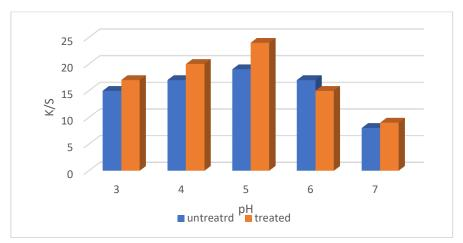
Figure 7. Effect of pH of the dye bath on K/S of wool fibers dyed by microwave
